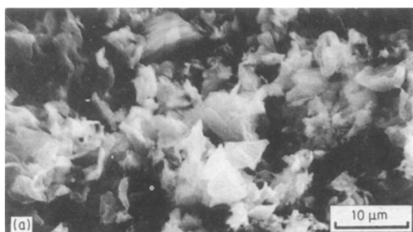
Figure 6 High magnification SEM image of the surface of oxidized graphite.
