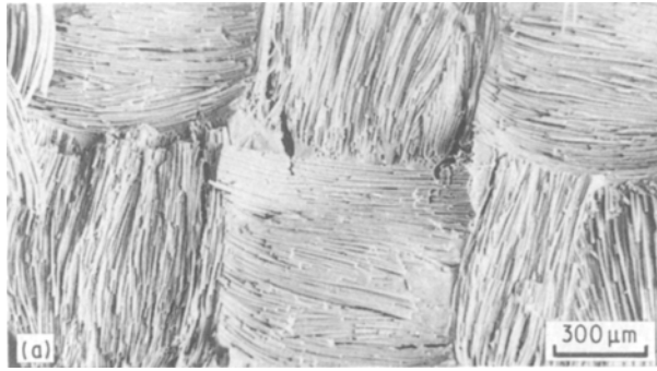
Figure 1 SEM micrographs of 2D fibre mat lay-up.
